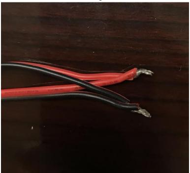
3. Insert the combined wires back to the connector, tighten the screws.
